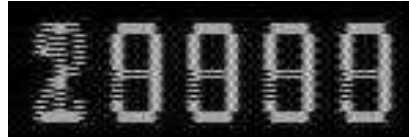
Figure 5. Superimposed frame numbers on a frame are output frame numbers from eye-tracker which are superimposed on a frame. This figure shows the worst-case scenario where two frame numbers are overlapped on the same frame.
