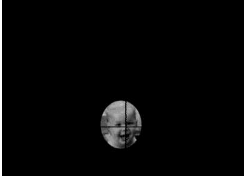
Figure 4. The reference image is an image which represents the image displayed in between the trials. We are able to find the start and end frame for each trial by calculating the correlation between the current frame and this reference image. If the correlation is less than 0.8 then we have detected the start frame.
